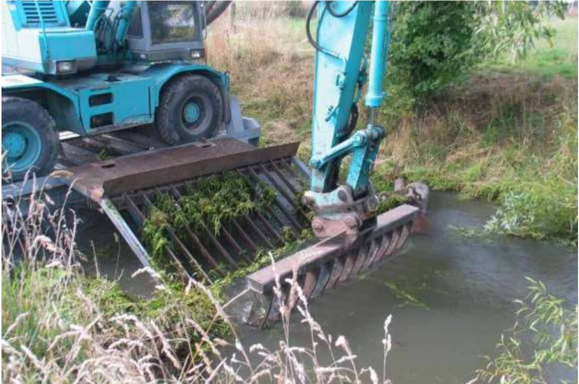
Figure 26 Rake bucket used in the Waimakariri District for aquatic weed removal
