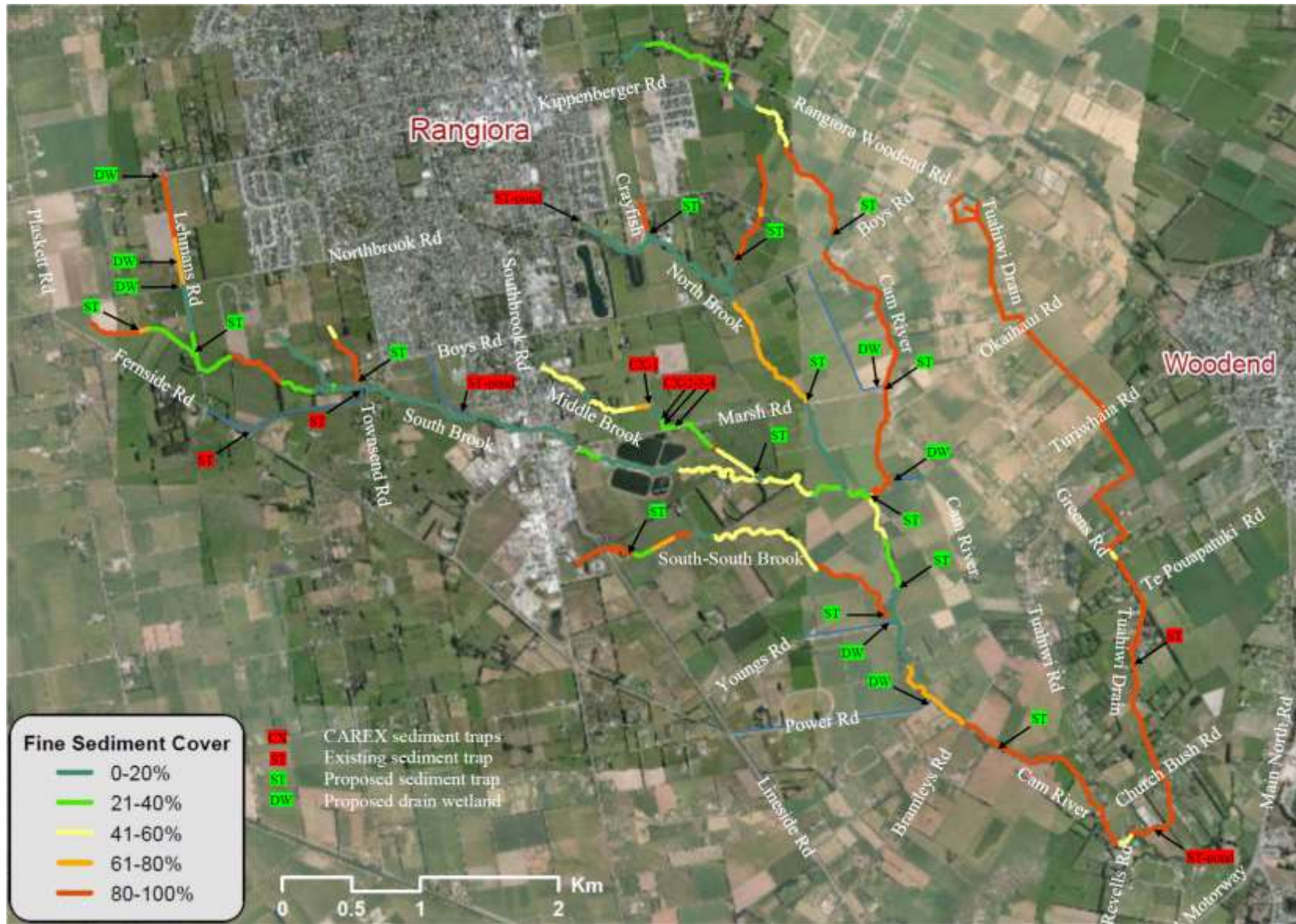
Figure 5 Fine sediment cover (map kindly provided by ECan) proposed & existing sediment traps & drain wetlands
