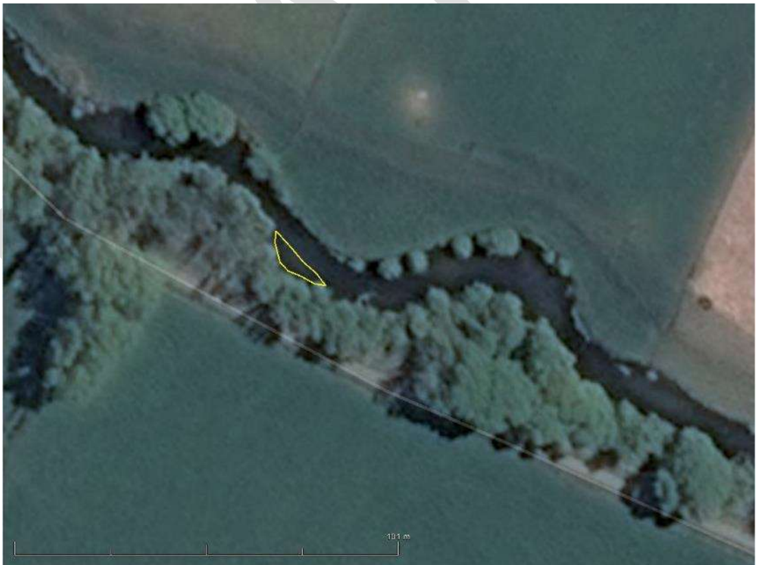
Figure 17 Natural sediment deposition areas can be utilised as sediment traps by removing sediment to revitalise deposition (Cam River ~300 m below Bramleys Road)
